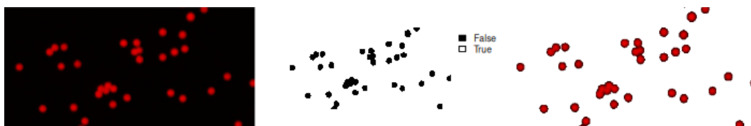
Figure 5: Displaying the original, background, and foreground Images: The original image (left) shows the fluorescent microbeads. The middle image displays the background in white (TRUE) and all objects detected by segmentation in black (FALSE). The right image shows only the foreground (microbeads) after detection through segmentation using the fieldMASK() function.
