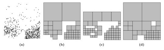
Figure 7: Examples of the effect of the ineq.threshold parameter. a) Subset of points used in the example; b) AQuadtree with default ineq.threshold value; c) AQuadtree with ineq.threshold value 0.01; d) AQuadtree with ineq.threshold value 0.5.
