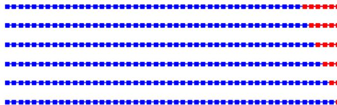
**Figure 9:** Training (blue) and test (red) sets for rolling origin evaluation with 6 observations.
