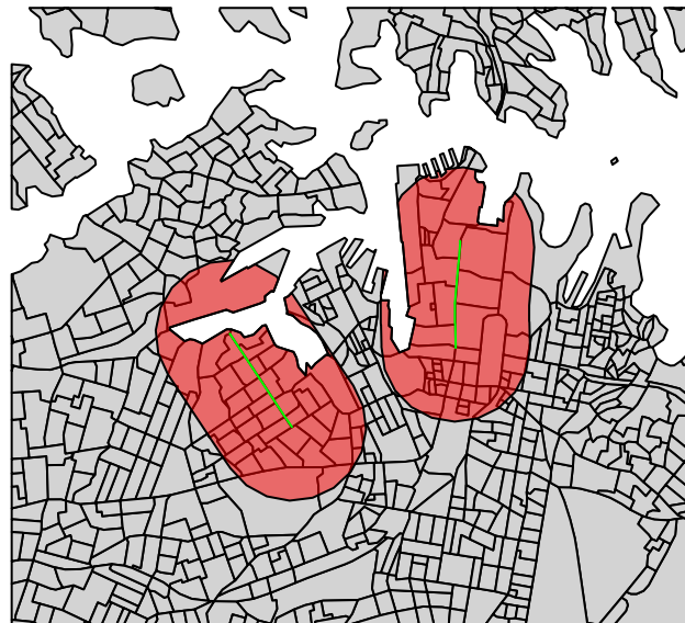
Figure 5: An 800 metre catchment area (red) associated with a cycle path (green) using straight-line distance in Sydney.
