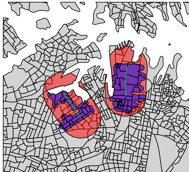
Figure 6: A 800 metre network catchment area (blue) compared with a catchment area based on Euclidean distance (red) associated with a cycle path (green).
