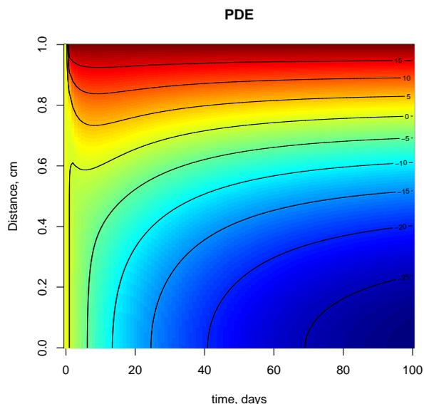
Figure 6: Dynamic solution of the 1-D diffusion-reaction model.
