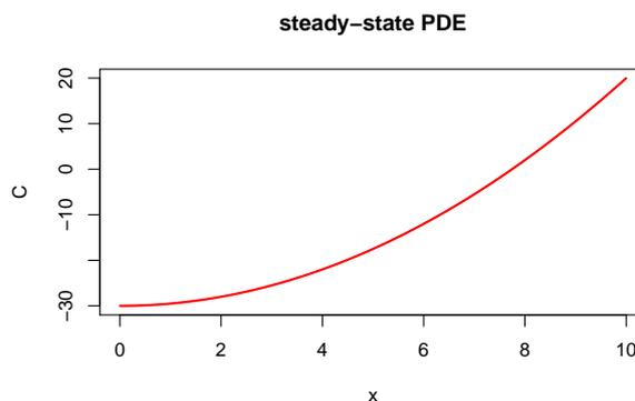
Figure 5: Steady-state solution of the 1-D diffusion-reaction model.
