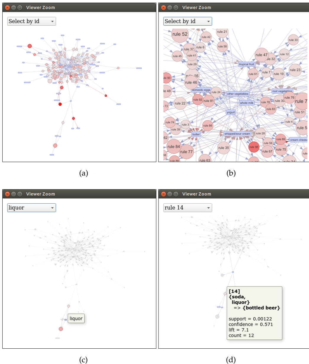
Figure 7: Graph-based visualization with items and rules as vertices. Plot (a) shows the initial view of the complete graph. Plot (b) uses zooming in to show the center of the graph, revealing the most frequent items (including “other vegetables” and “milk”). Plot (c) shows how to use the pull-down menu in the top-left corner to find the item “liquor” in the graph. Plot (d) inspects a single rule that is connected to “liquor.”
