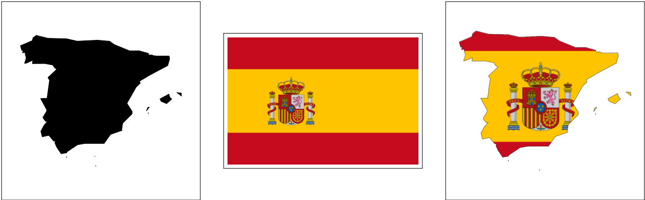
Figure 12: A raster image of the Spanish flag being used as a fill pattern for a map of Spain. On the left is a map of Spain filled in black (produced by the map() function from the maps package). In the middle is a PNG image of Spanish flag (a public domain image from Wikimedia Commons, http://en.wikipedia.org/wiki/File:Flag_of_Spain.svg ), and on the right is the result of clipping the Spanish flag image using the map as a mask.
