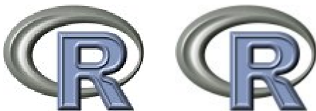
Figure 6: The R logo drawn using the old behaviour of drawing a small rectangle for each pixel (left) and using the new raster support with linear interpolation (right), which produces a smoother result.
